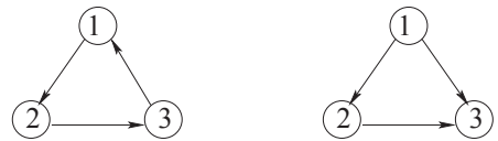
Fig. 4. Two non-isomorphic directed graphs with three nodes
