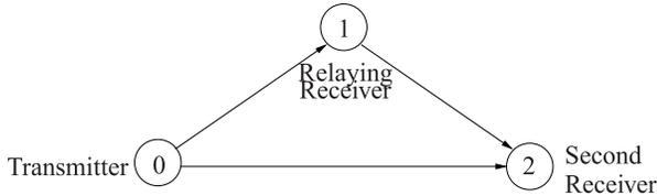
Fig. 1. The relaying broadcast channel.
