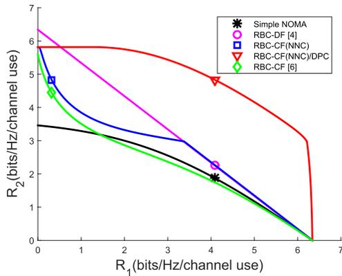
Fig. 3. The achievable rate region for a component channel.
