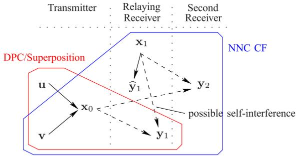
Fig. 2. Markov chain relationship between codewords and received signals (solid arrows: codeword Markov chain and dashed arrows: channel links).
